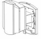
Step 6: Mount the light - Snap the indication light onto the mounting plate. You will hear a "click" when the light is securely in place.
