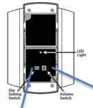
Step 2: Select settings – Remove front lens using a 2mm flat-head screwdriver and select light settings. The dip switches control whether the ILB-21 will forward alarms to a central monitor unit or as a night light. The buzzer volume is adjustable from 89-108dB.
